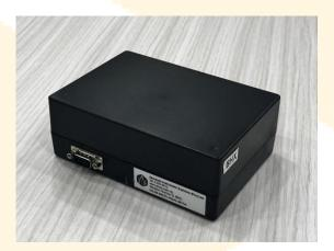
NT326 is used to convert serial RS232 interface equipment to a Modbus RTU interface.
